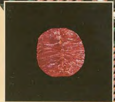
Typical cast anode with large grain structure
